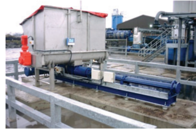
A seepex BTE 35-48 pump fitted with a live bottom storage silo receiving off specification sludge for reprocessing. Sludge is loaded into the pump hopper via a front loader. Storage capacity: 6 m 3 .
